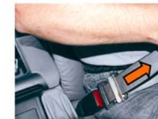
8. Buckle up as usual, then simply pull the slack out of the lap belt by pulling the shoulder belt as shown by the red arrow. If you need more slack to buckle up, depress the lever to let the seatbelt slide through the CG-Lock.
